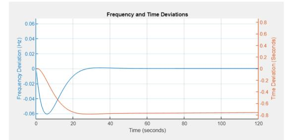
Figure 5: Frequency and Time Deviation Trajectories - Single Initial Disturbance
