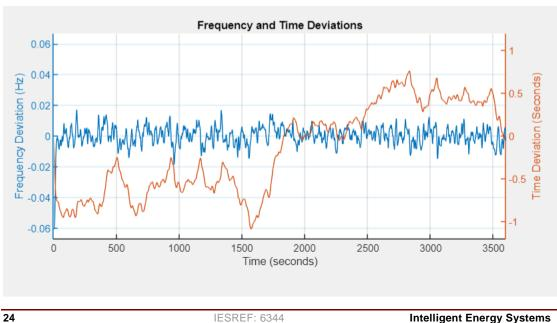
Figure 7 : Frequency and Time Deviation Trajectories over a One-hour Period
