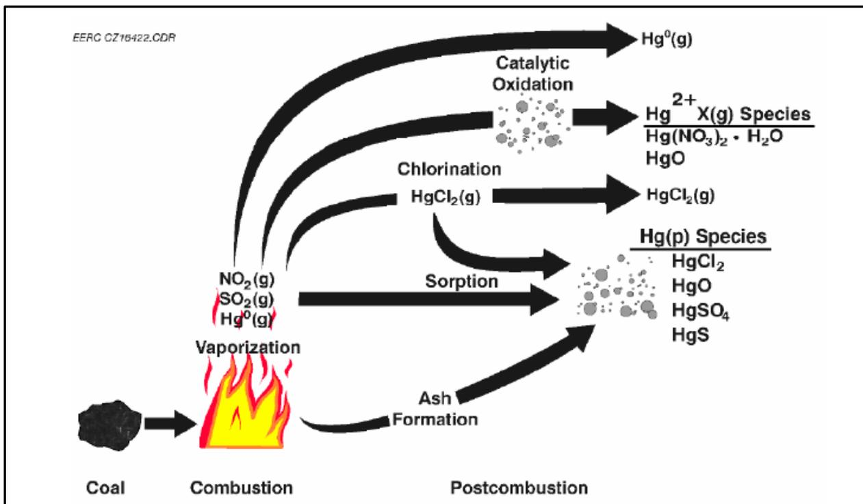
**Figure 7 Potential Mercury Speciation Pathways from Coal Combustion (Newman-Sutherland et al. 2001)**
